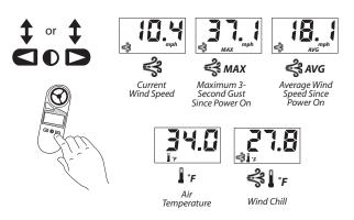
4) Select the units of measure. Press ▶ while holding ● to scroll through the units of measure.
