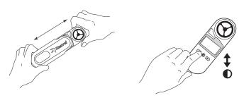
Select operating mode. Press the right arrow (▶) to scroll through the measurements listed below. Press the left arrow (◄) to scroll through the measurements in reverse order. The instantaneous measurements will be displayed. (See Understanding the Measurements section for more information.)
