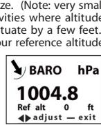
which use satellite triangulation to determine altitude. Note that with present GPS technology, pressure altimeters remain more accurate for measuring altitude change. This is why airplanes still rely on pressure altimeters, not GPS. Finally, the DENSITY ALTITUDE screen is calculated from the absolute values of station pressure, relative humidity and temperature, and is not affected by the reference values entered in the BARO and ALTITUDE screens.
