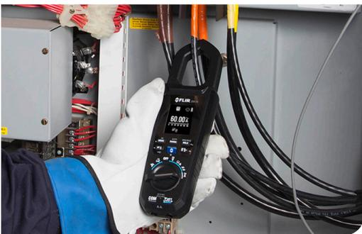
Verify amperage measurements
