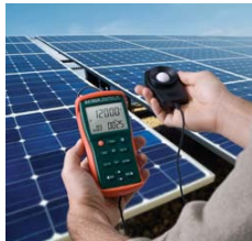
Wide range for taking measurements in direct sunlight
