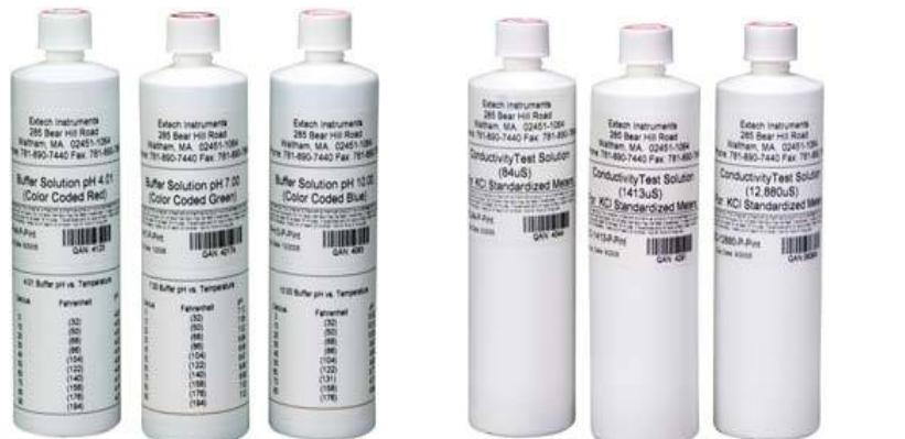
Pint size pH buffers for pH 4, 7, and 10 available EC-84-P, EC-1413-P, and EC-12880-P pint size conductivity standards (PH4-P, PH7-P, PH10-P)
